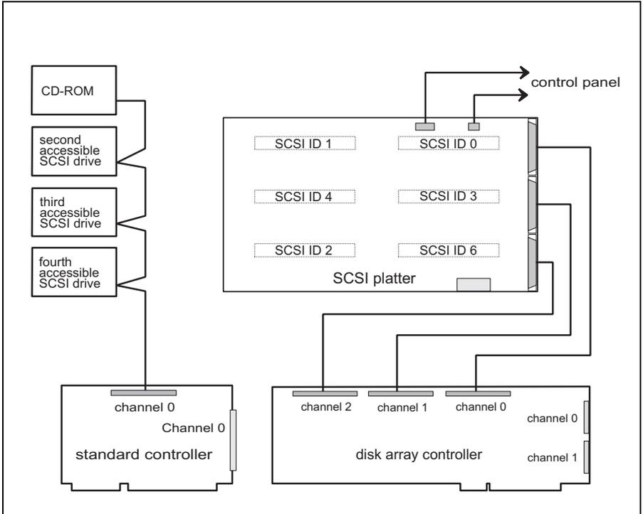
Cabling of disk array controller and standard SCSI controller
