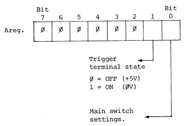
Ø: Main switch is set to OFF.1: Main switch is set to ON.
