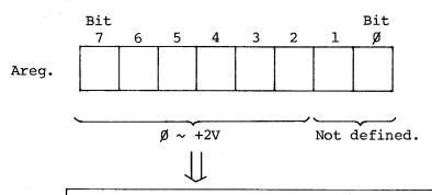
Each bit corresponds to  $2V \div 2^6 = 32mV$ . These bits are all set to 1 when a voltage higher than +2V is input. They are set to  $\emptyset$  when a negative voltage is input.
