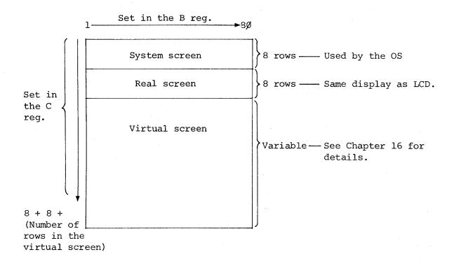
RDVRAM reads the number of characters specified by DE starting at the position designated by B and C and stores them sequentially into the area starting at the address designated by DE. Characters are read from left to right in a row. After the 80th character is read, the leftmost character in the next row is read.
