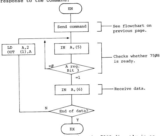
Points to be noted when using the 7508 directly in an application program
