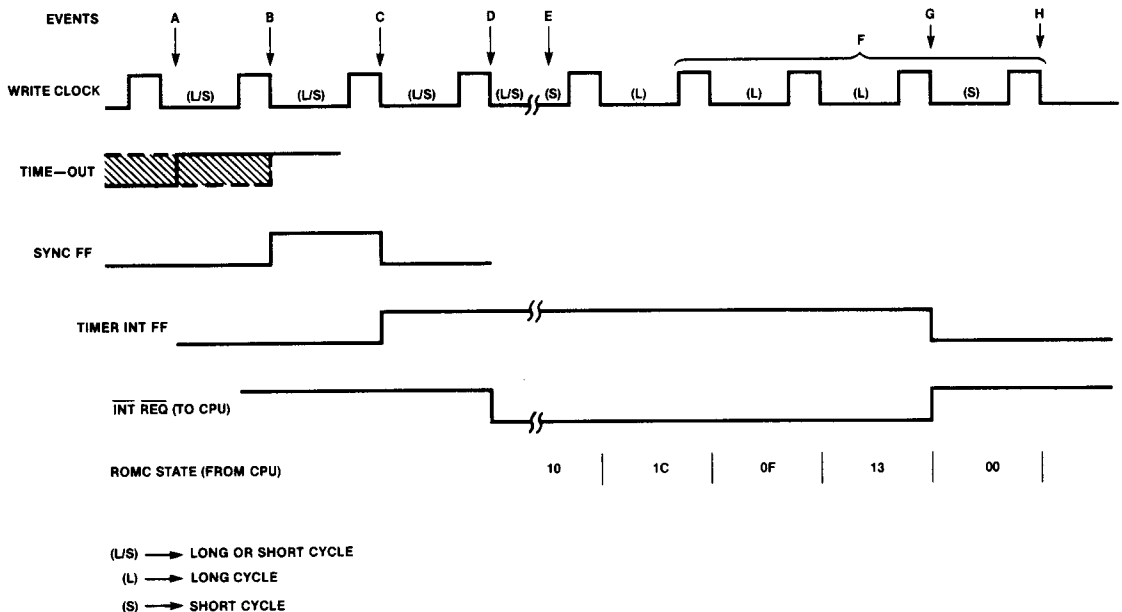
Figure 15 Timer Interrupt Sequence
