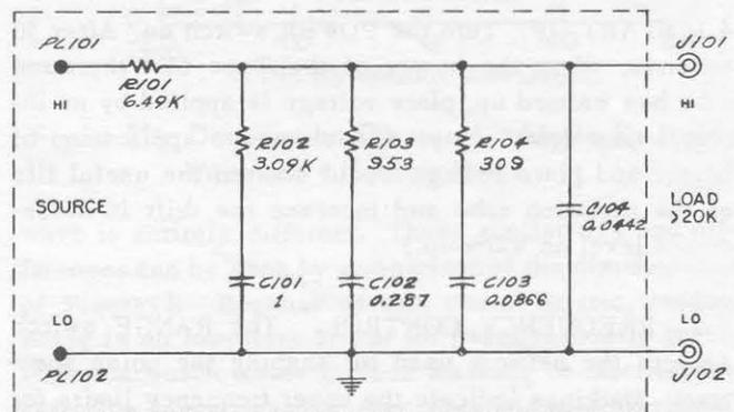
Figure 10. Schematic diagram of the Pink-Noise Filter.
