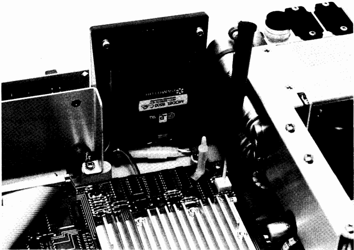
Figure 3-3 Adjusting the Clock Frequency
