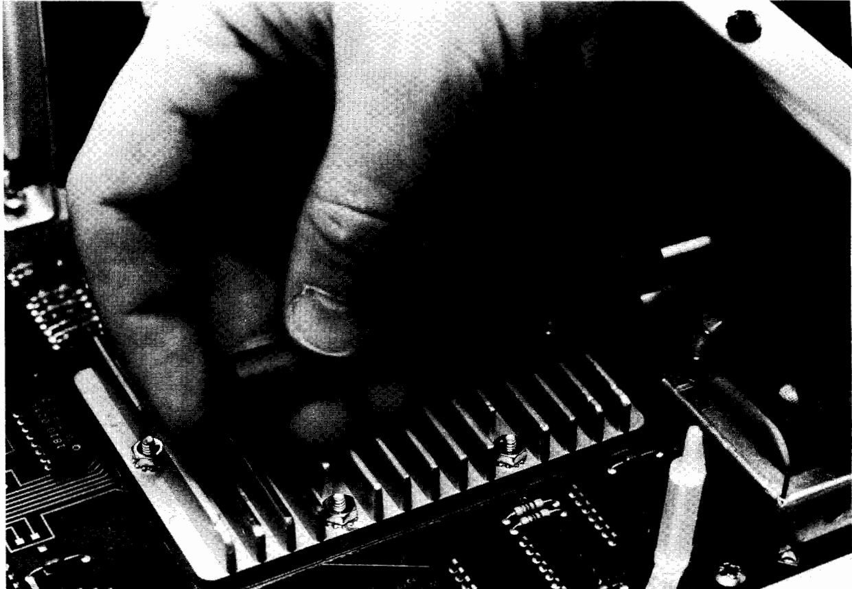
Figure 3-2 Adjusting the +12 Volt Supply
