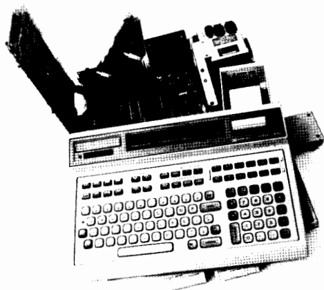
Fig. 1. 9825A Calculator is fully operational when opened for servicing. Printed circuit boards are hinged to provide access to both sides. Plug-in ROMs at front and side were pulled halfway out for this photo.
