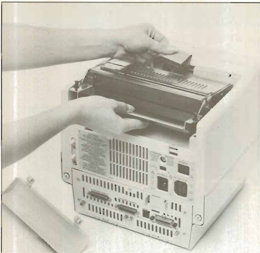
Photo 1: A back view of the HP 150. Note the two serial ports (DATACOM1 and DATACOM2), the port for HP-IB bus (used to connect a series of disk drives and parallel printers), and the easily removed battery.
