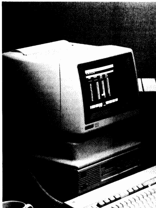
Fig. 1. The 2674A Printer is a thermal printer that fits into the top of the HP 150 Personal Computer cabinet.
