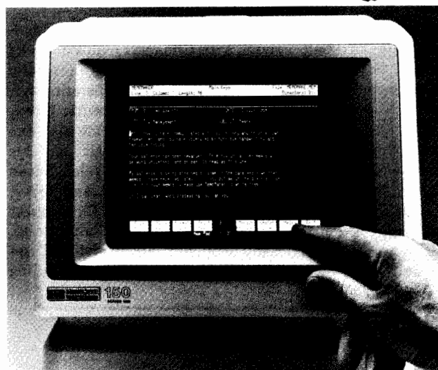
Fig. 3. The green-phosphor CRT displays 24 80-character rows of text, plus three rows of status and softkey information.
