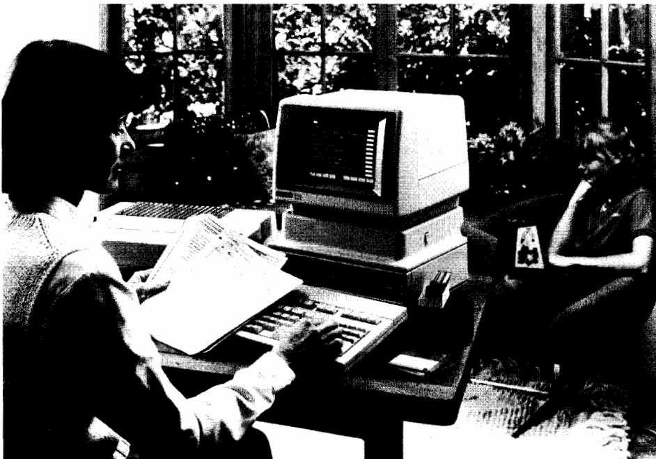
Fig. 1. The HP 150 Touchscreen Personal Computer consists of three modules: a system processing unit with integral display, a disc unit, and a keyboard. Without the disc unit, it operates as an HP graphics terminal.
