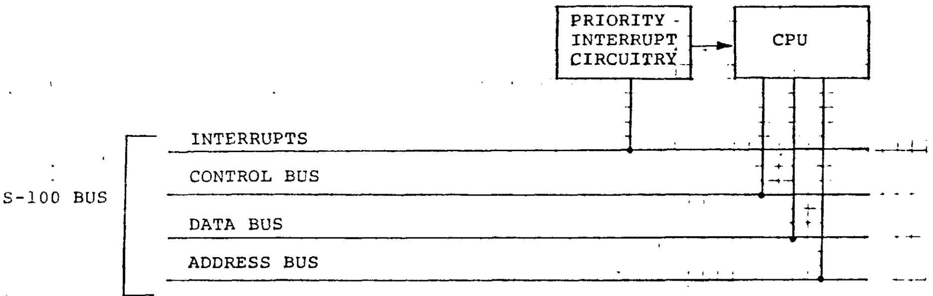
FIGURE 2 - I/O BOARD BLOCK DIAGRAM
