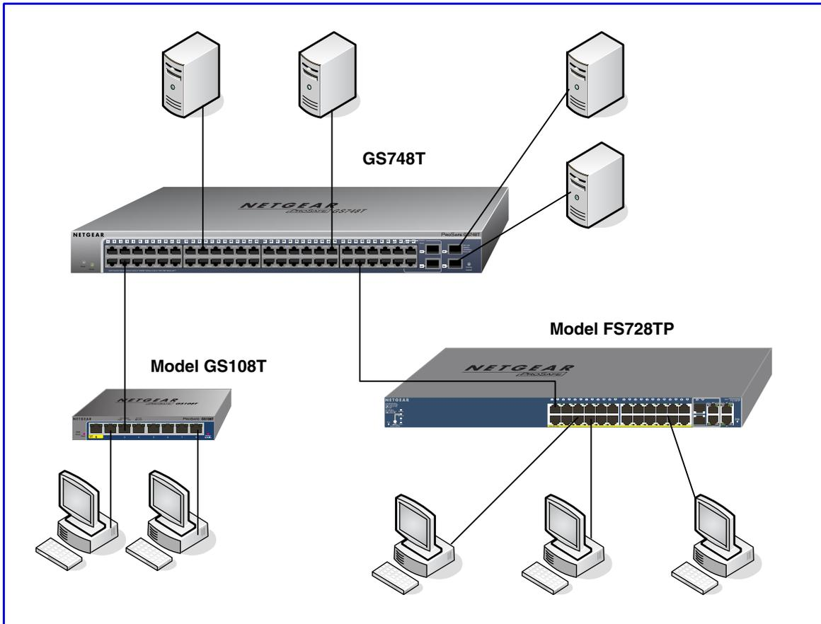
Figure 5. Backbone Switching
