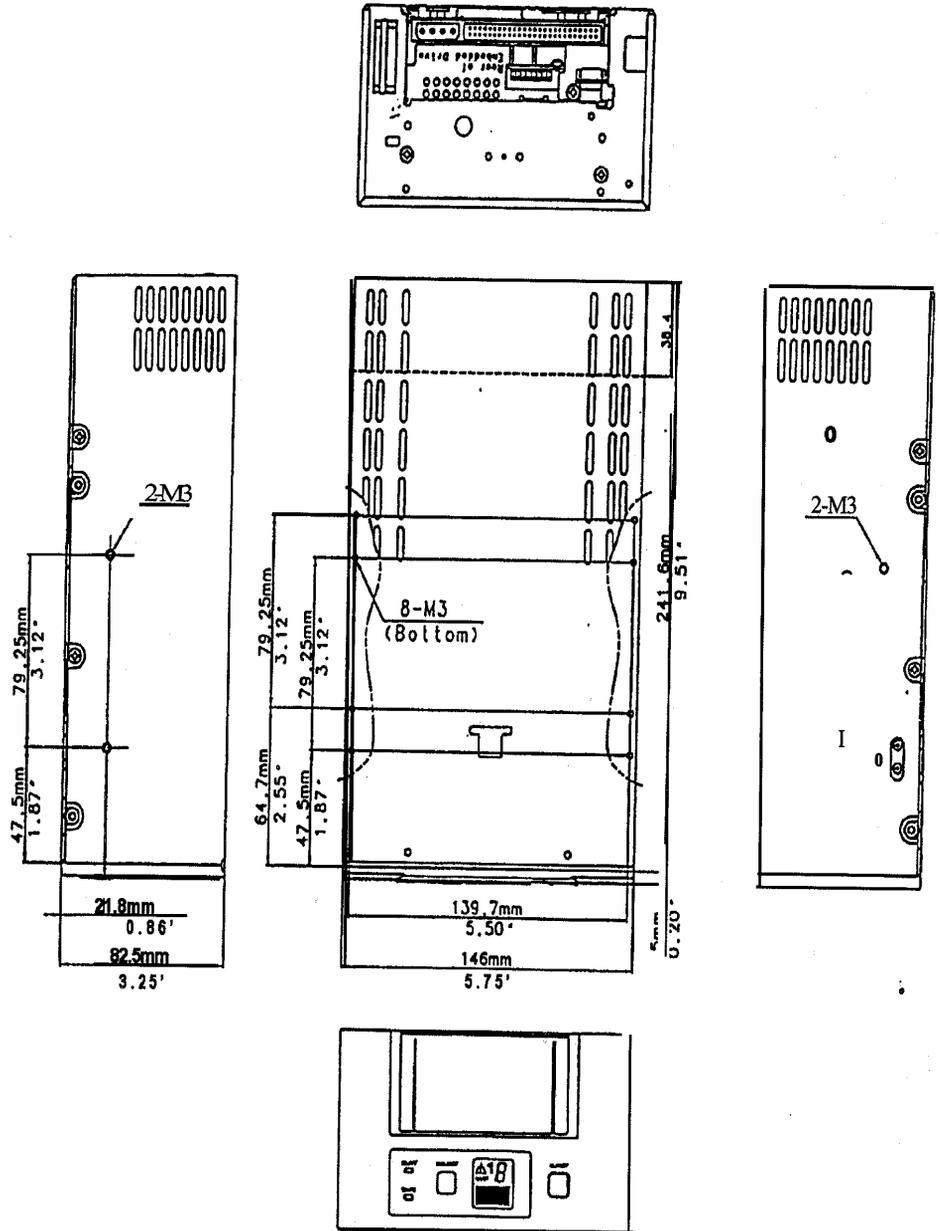
Figure 2-5. Mounting Holes 5.25-inch autoloader (Internal)
