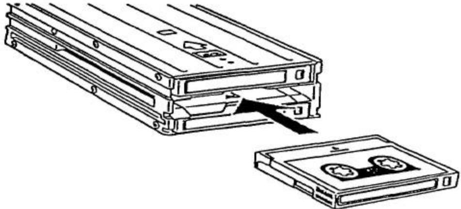
**Figure 3-8. Inserting a cartridge into the middle magazine shelf**
