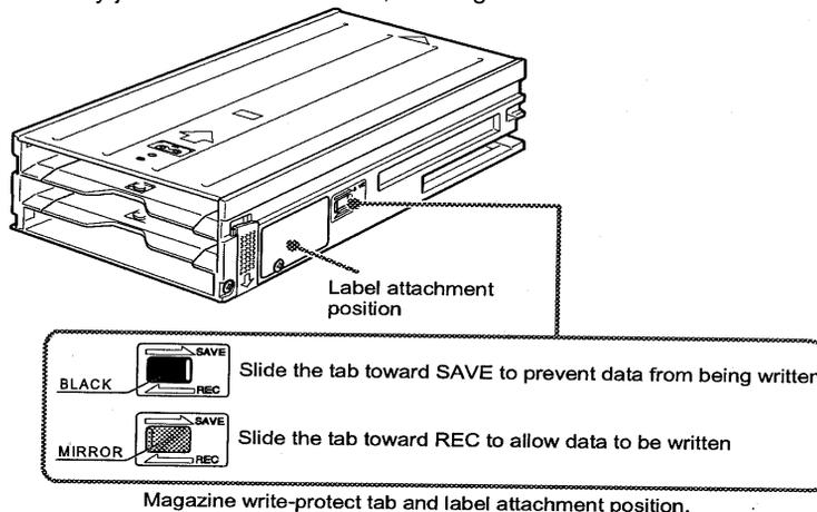
**Figure 3-13. Slide Stopper, Write Protect and Index Label**
