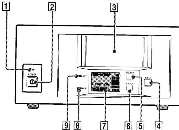
**Figure 2-1. Front Panel (External)**
