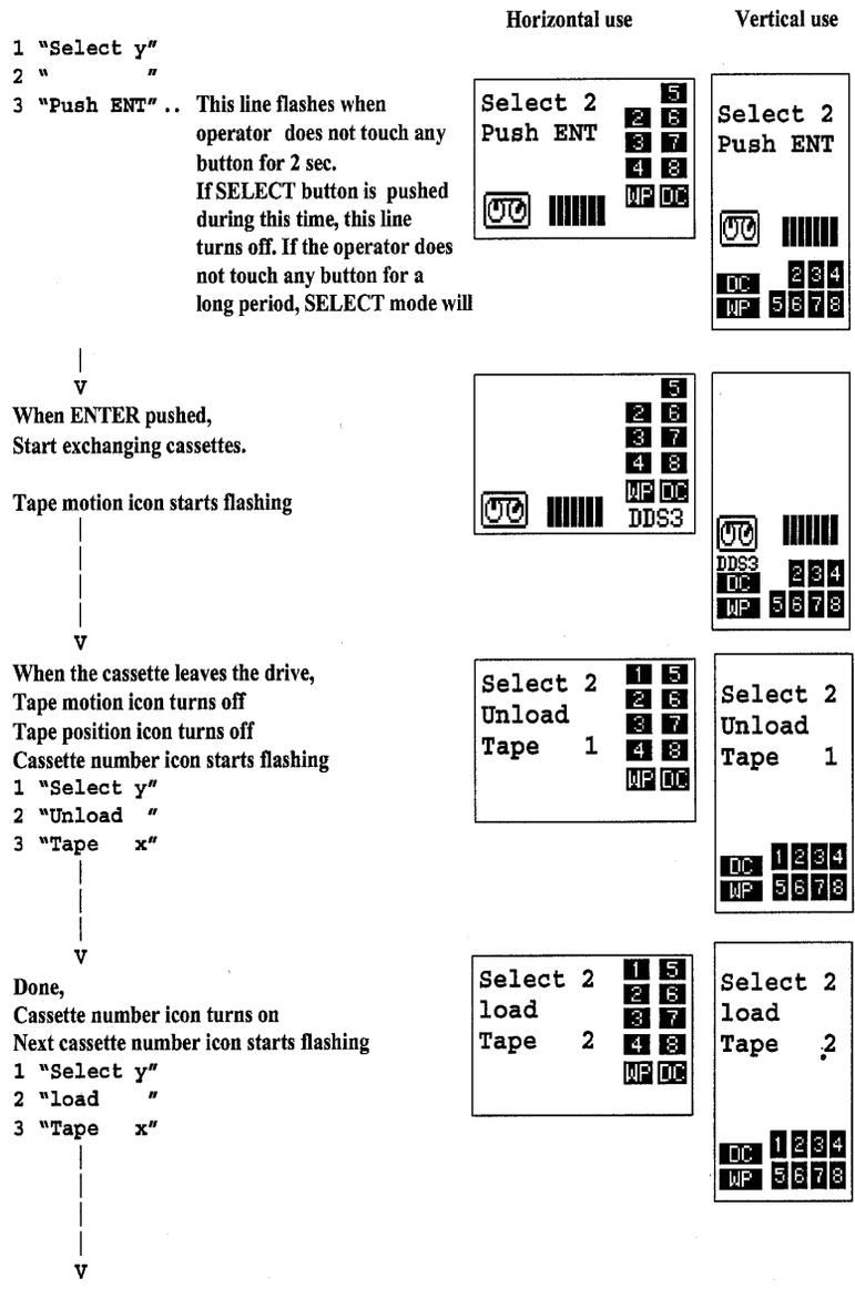
Figure A-12. Select and Load Tape
