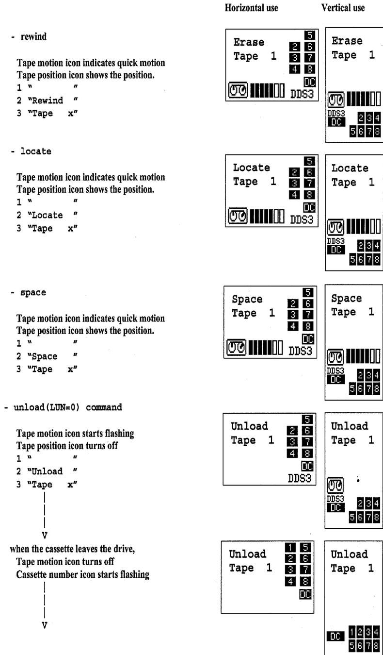
Figure A-8. Erase, Locate Tape, Space Tape, Unload Tape
