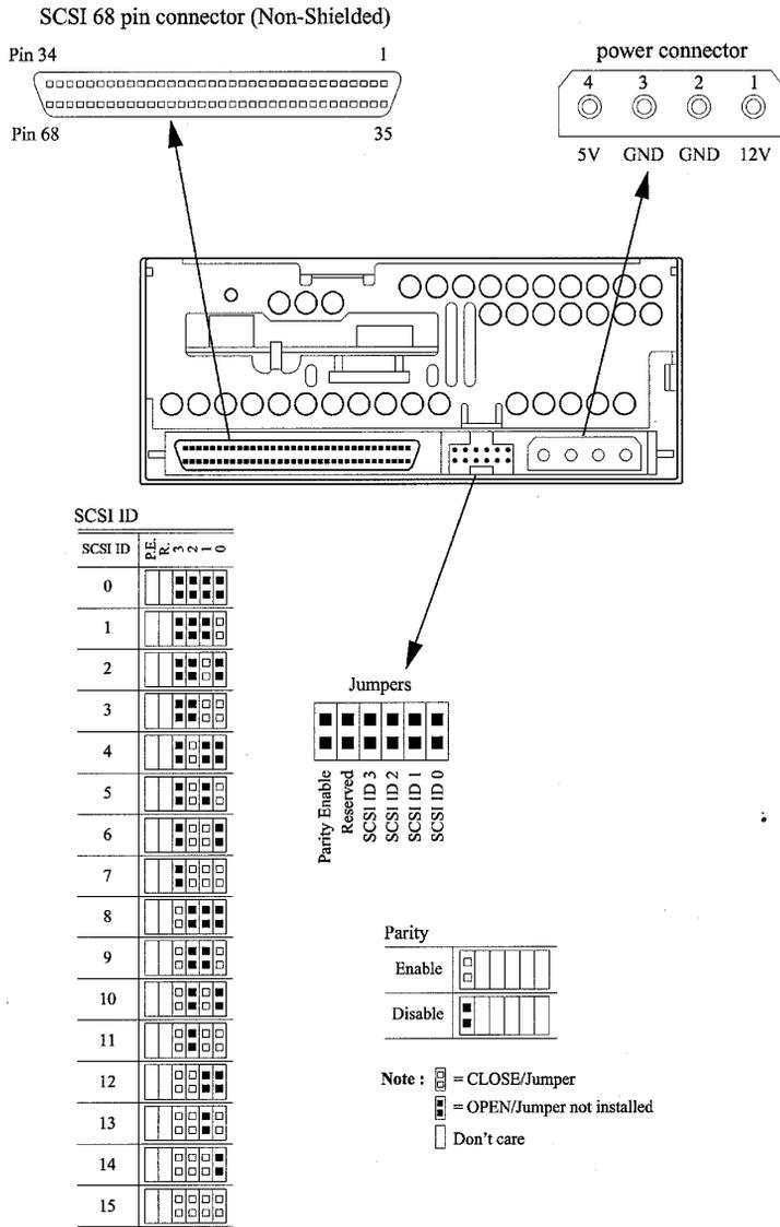
**Figure 2-3. Rear Connectors and Jumpers (Internal)**
