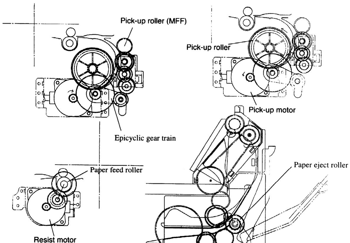
**Figure 5-3 Structure of the Paper Feed Drive Unit**
