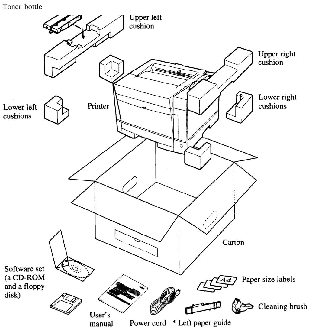
**Figure 2-1 Shipping Carton and Printer and its Accessories**
