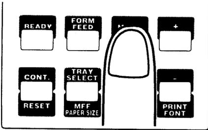
**Press the MENU button to put the printer in menu mode.**
