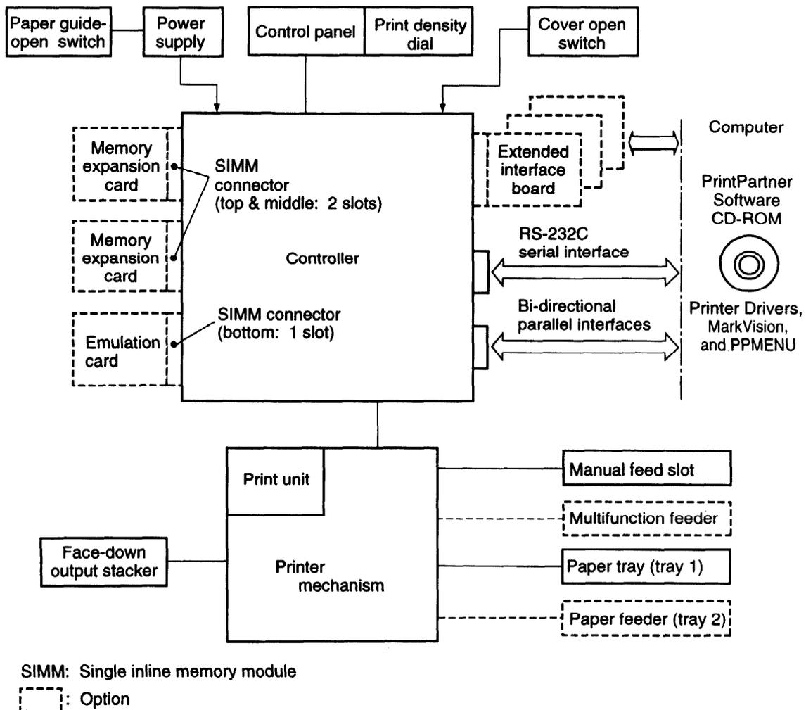
Figure 5-1 Printer Block Diagram
