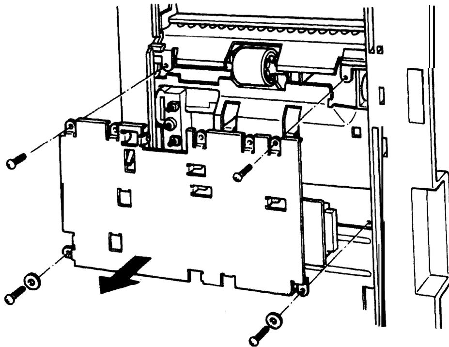
Remove six screws to remove the sensor board assembly.
