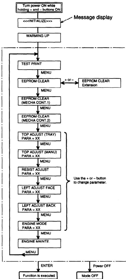
1. Turn on the power switch while pressing and holding down the + and - buttons until the message display indicates TEST PRINT. (It takes about one minute, but depends on warming-up time.)
