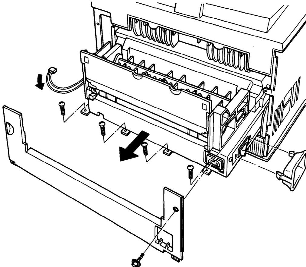
Disconnect the two connectors while pressing the connector lock with a standard screw driver as shown below. (The following illustration shows the side that faced to the front of the printer when the unit was installed.)
