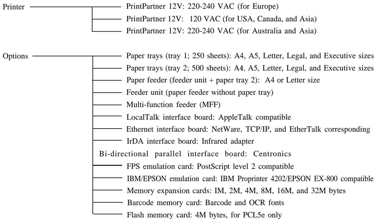
The standard printer has 4 megabytes of RAM, an HP LaserJet 5 (PCL6) emulation, a Centronics parallel interface (bi-directional), and an RS-232C serial interface. Its paper tray size is A4 for Europe and Asia, and letter for USA, Canada, and Australia.
