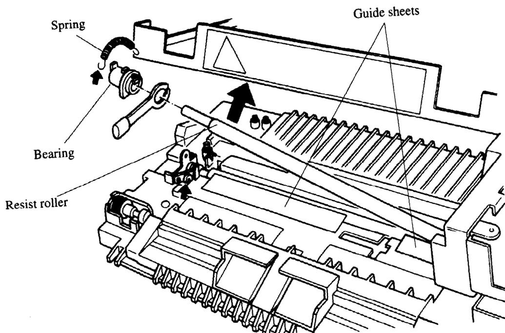
Cut the hook of the gear at the right end of the paper feed roller using a diagonal cutting pliers, Move the paper feed roller to the left and pull out the roller from the left end.
