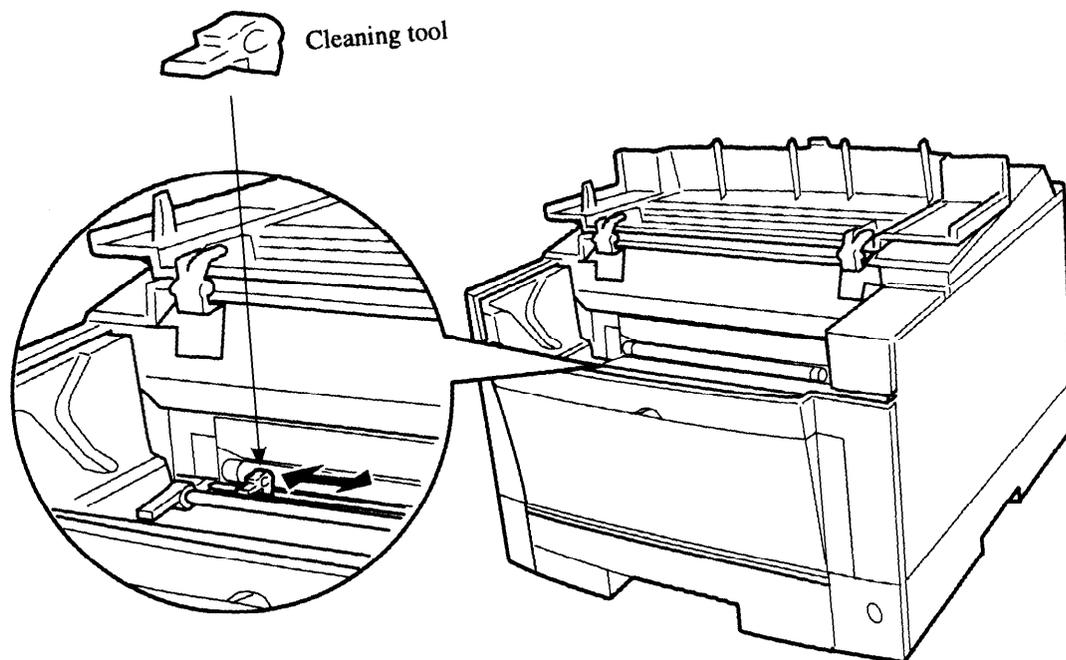
**Figure 4-3 Cleaning the Corona Wire**
