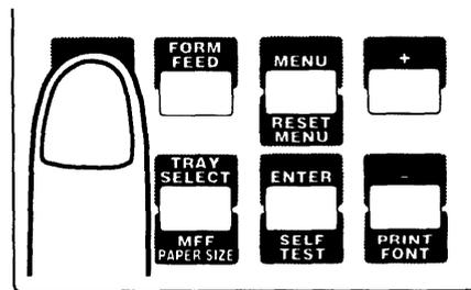
Press the READY button to return the printer online. The ONLINE indicator lights up without the REPLACE PARTS message
