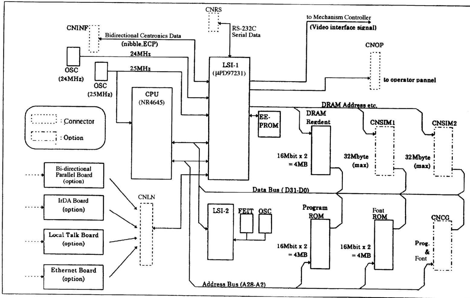
Figure 5-9 Control Board Block Diagram
