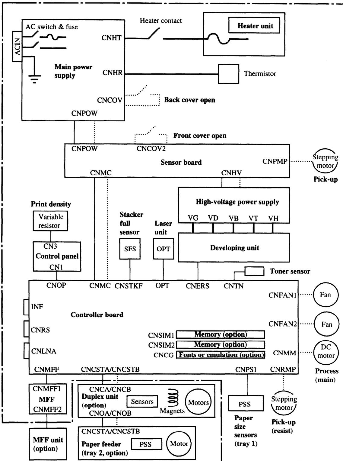
**Figure 3-1 Printer Elements and Connections**
