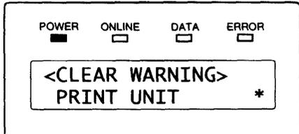
The message changes to <CLEAR WARNING> PRINT UNIT \*. The asterisk means that the print unit is expired.
