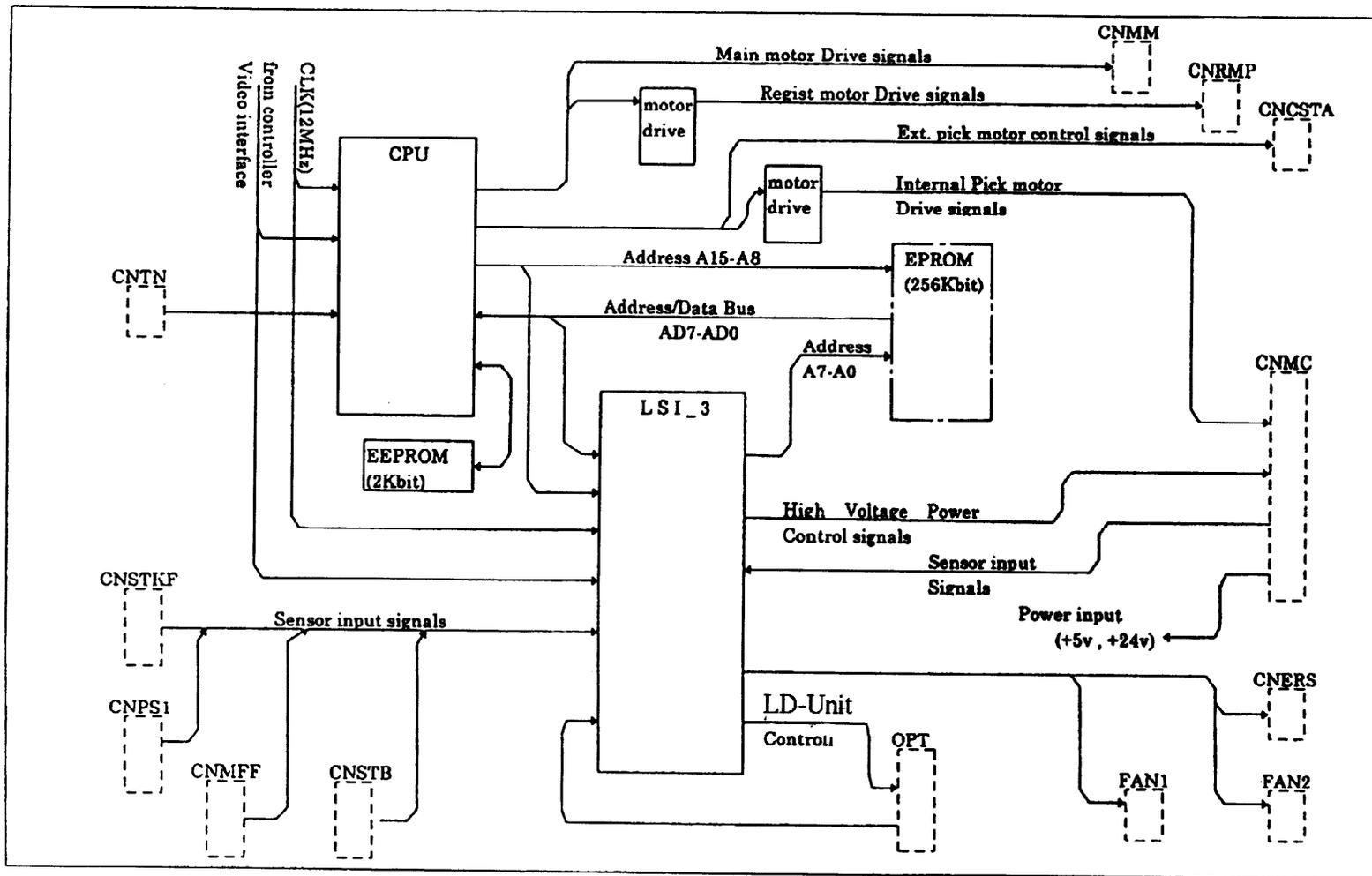
Figure 5-10 Engine Controller Block Diagram
