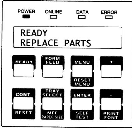
**Make sure the printer is offline.** If necessary, press the READY button to put the printer offline. The ONLINE indicator is off with the REPLACE PARTS message displayed.
