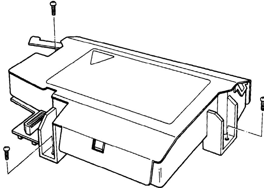
(Frame ground cover is removed from the top of the laser unit)
