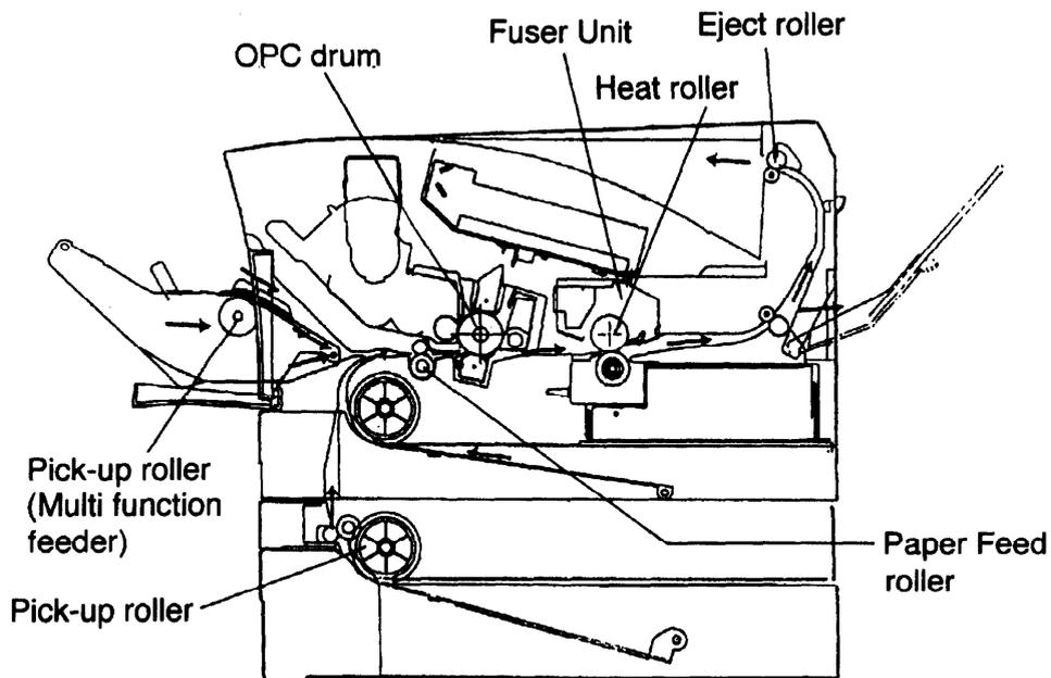
**Figure 5-2 Picking, Printing, Fusing, and Ejecting Paper**
