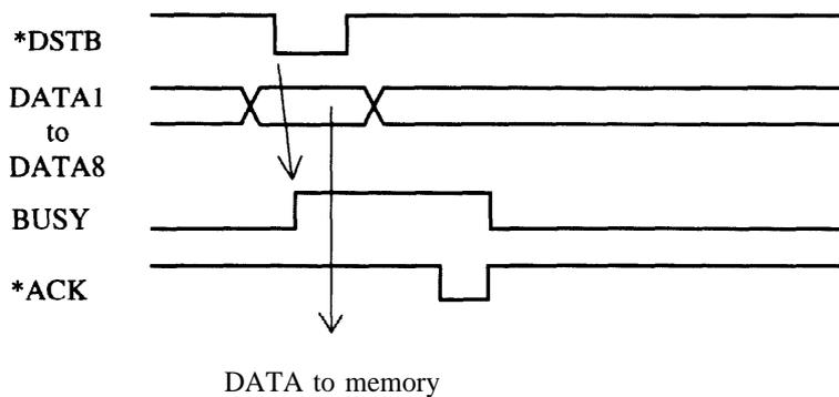
**Figure 5-11 Centronics Parallel Interface Signal Timing Chart**
