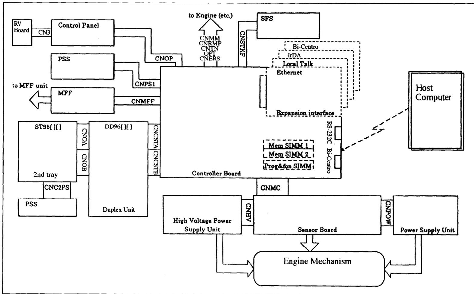
Figure 5-8 Main Controller Block Diagram
