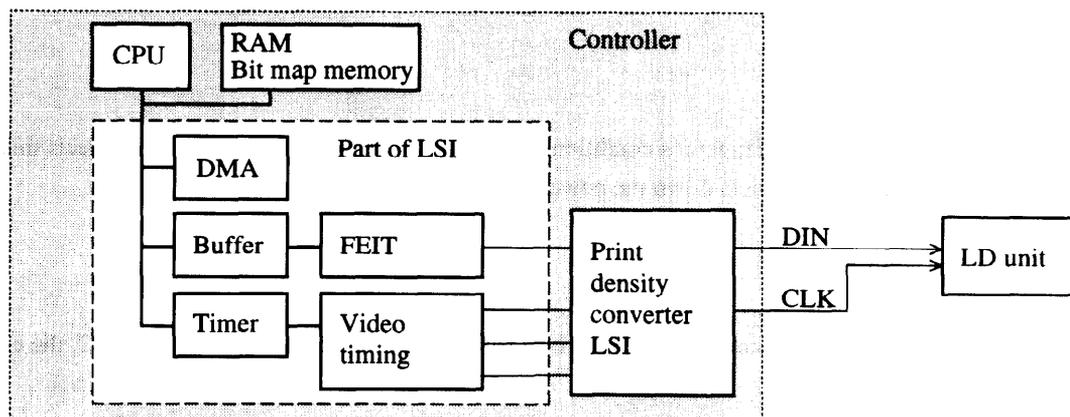
**Figure 5-15 Video Data Transfer Block Diagram**
