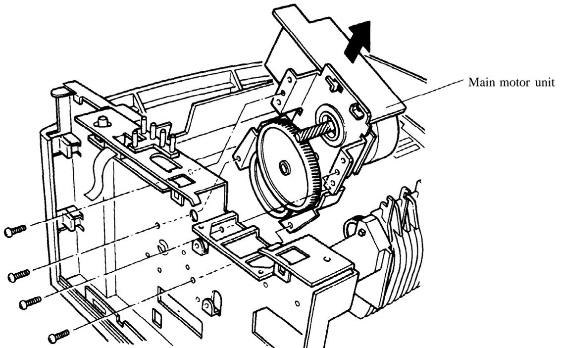
Remove four screws and disconnect the cable to remove the main motor.
