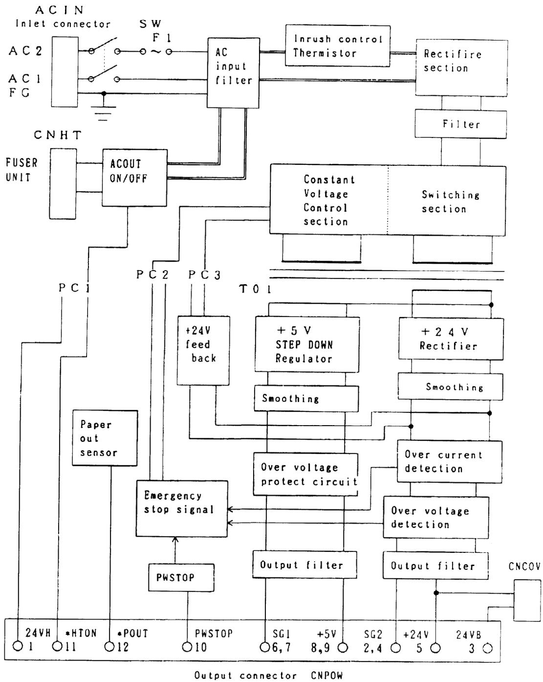
Figure 5-17 Power Supply Block Diagram
