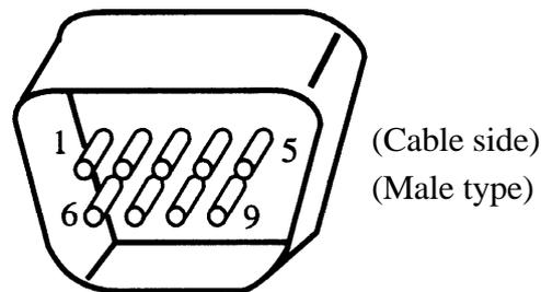
**Figure 5.7 Serial interface connector**
