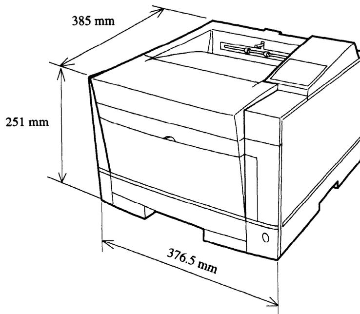
**Figure 1.2 Printer dimensions**
