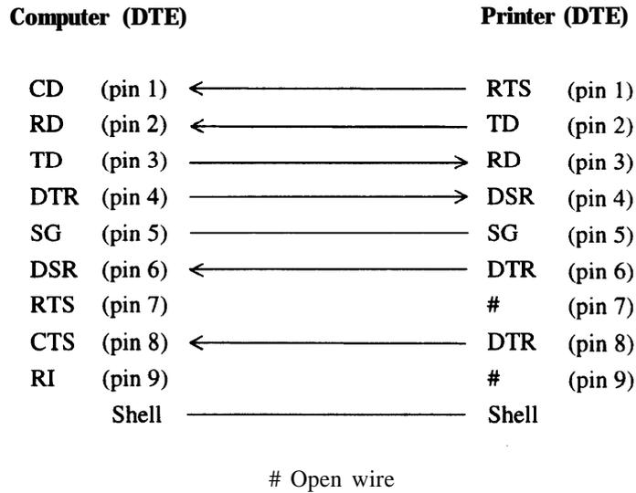
**Figure 5.9b Example of RS-232C cable wiring (9-pin connector at computer side)**
