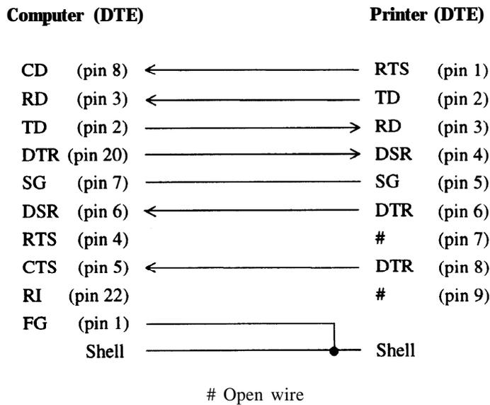
Figure 5.9a Example of RS-232C cable wiring (25-pin connector at computer side)
