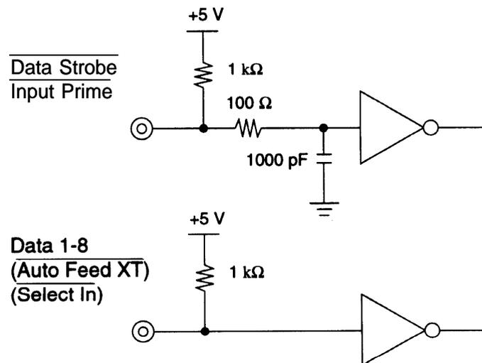
Figure 5.1 Parallel interface input circuit
