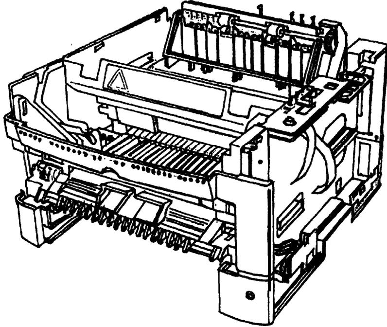
**Figure 2.4 Printer mechanism**
