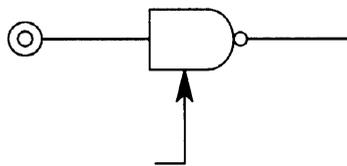
**Figure 5.5 RS-232C interface input circuit**
