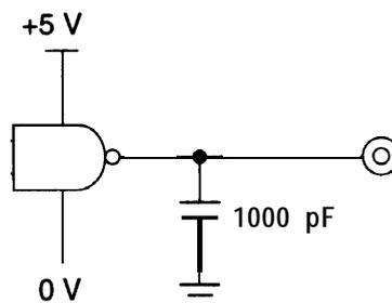
**Figure 5.6 RS-232C interface output circuit**
