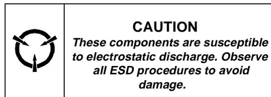
Semiconductor (solid state) devices that are easily damaged by static electricity are called Electrostatically Sensitive Devices. Examples are integrated circuits (ICs), large-scale integrated circuits (LSIs), semiconductor chip components, and some field-effect transistors.
