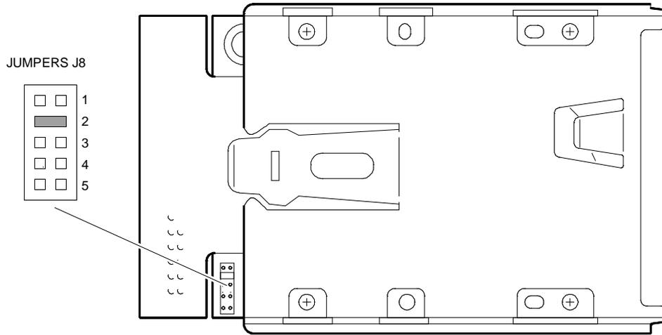
**Note:** Jumper J8 configuration is set at the factory and must not be modified.
