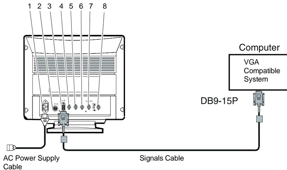
Fig. 1-2 Connection of the Signals and Power Supply Cables
