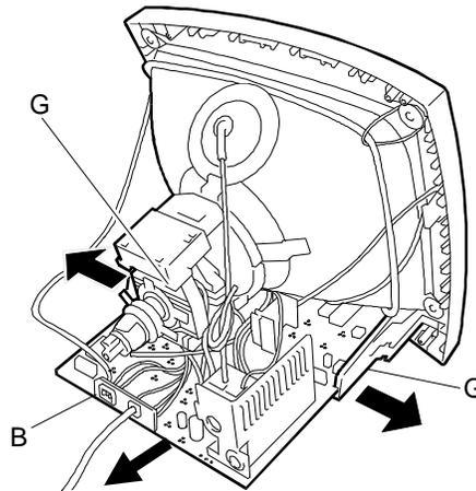
Fig. 2-9 Removing the Main Board
