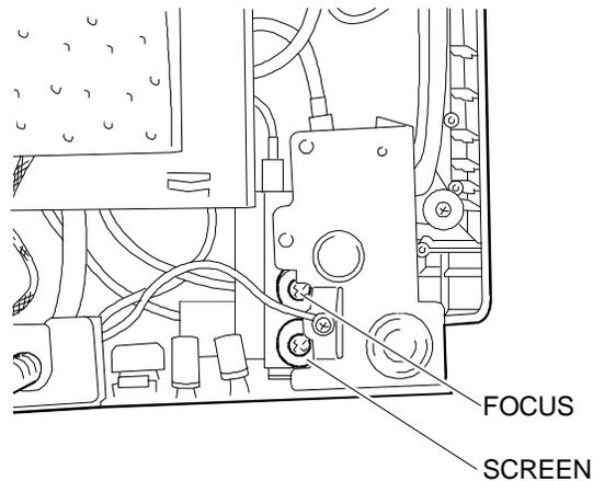
Fig. 2-16 Focus and Screen Potentiometers
