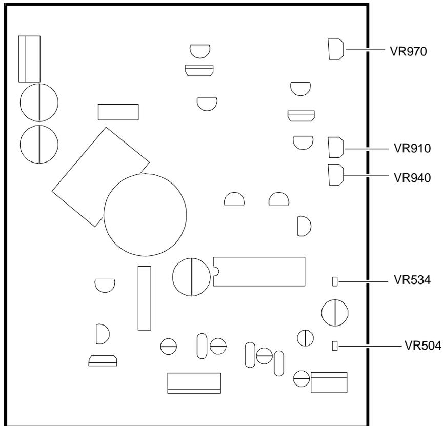
Fig. 2-14 Video Amplifier Board Adjustments
