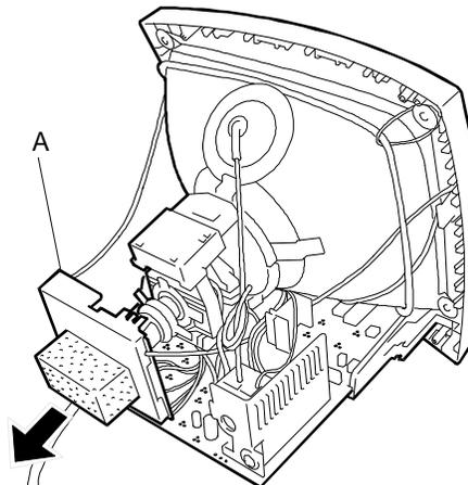
Fig. 2-7 Removing the Video Amplifier Board
