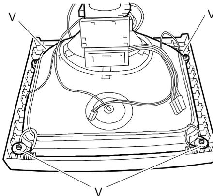
Fig. 2-11 Removing the CRT
