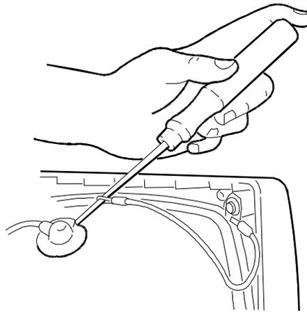
Fig. 2-5 Discharging the CRT Anode
