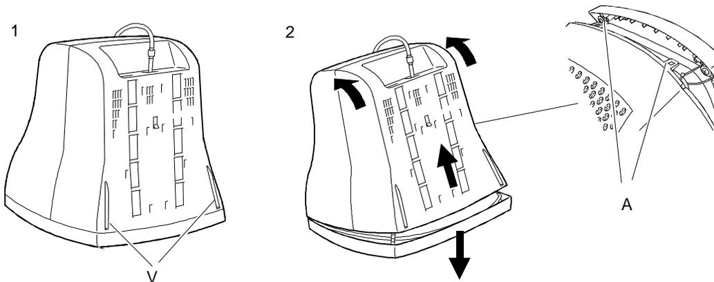
Fig. 2-4 Removing the Monitor Case
