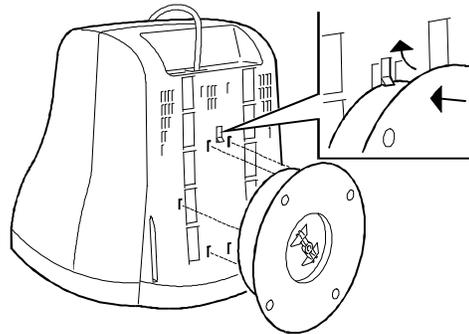
**NOTE:** During this operation be careful not to damage the monitor case securing holes.
