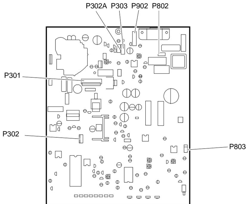
Fig. 2-10 Locating the Connectors on the Main Board
