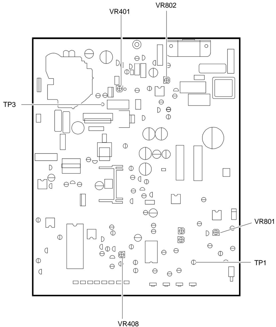
Fig. 2-15 Main Board Adjustments
