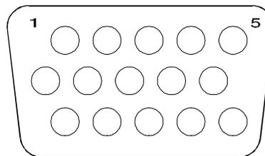
Fig. 2-1 DDC-1/2B VGA Connector
