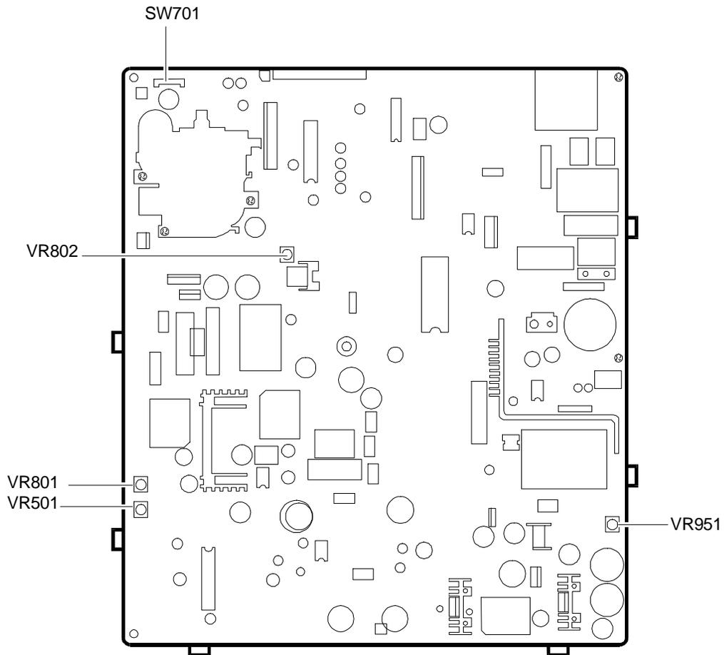
Fig. 3-18 Main Board Adjustments
