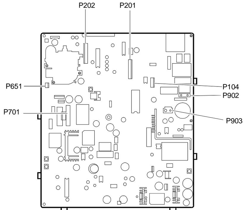
Fig. 3-9 Locating the Connectors on the Main Board
