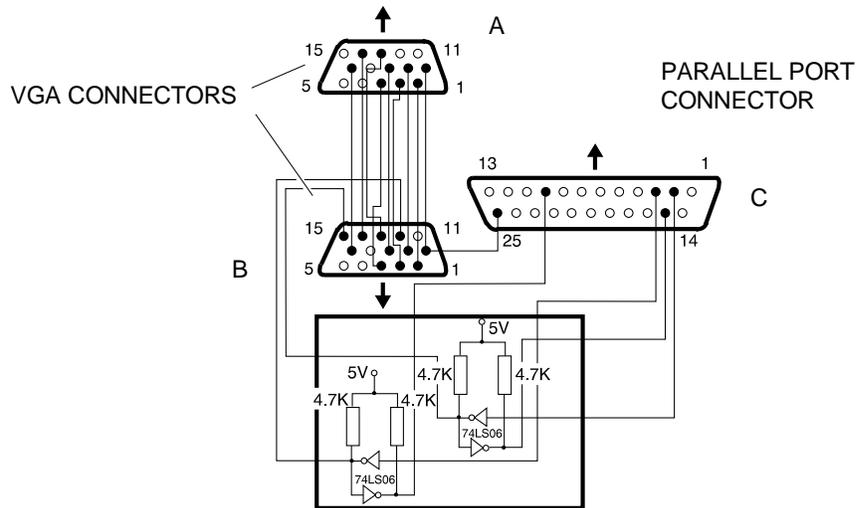
Fig. 3-21 Adapter Cabling
