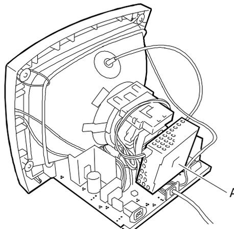
Fig. 3-7 Removing the Video Amplifier Board
