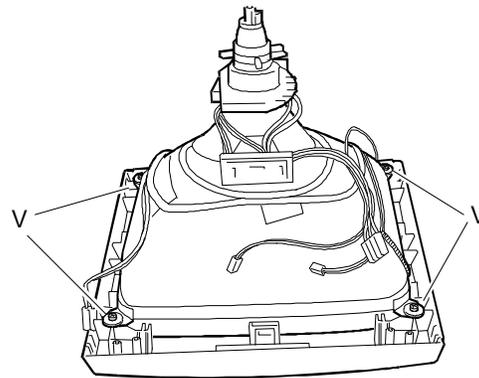
Fig. 3-14 Removing the CRT
