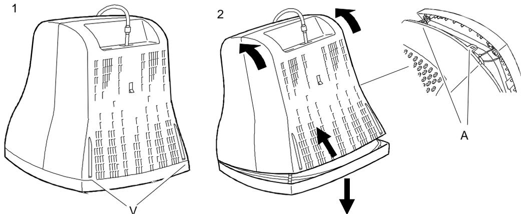
Fig. 3-4 Removing the Monitor Case
