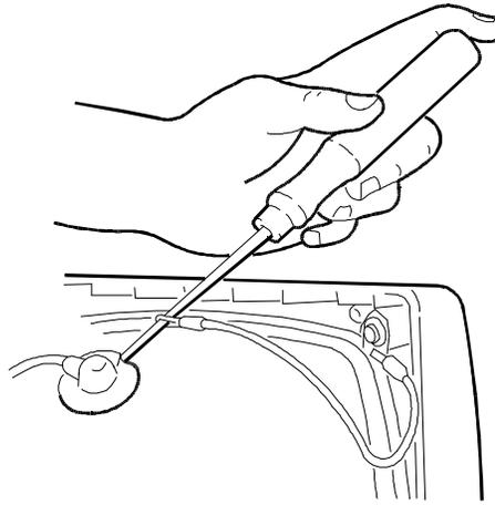
Fig. 3-5 Discharging the CRT Anode
