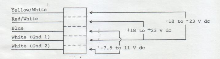
Figure 2-7. Sol-20 power connector and voltage measurements.
