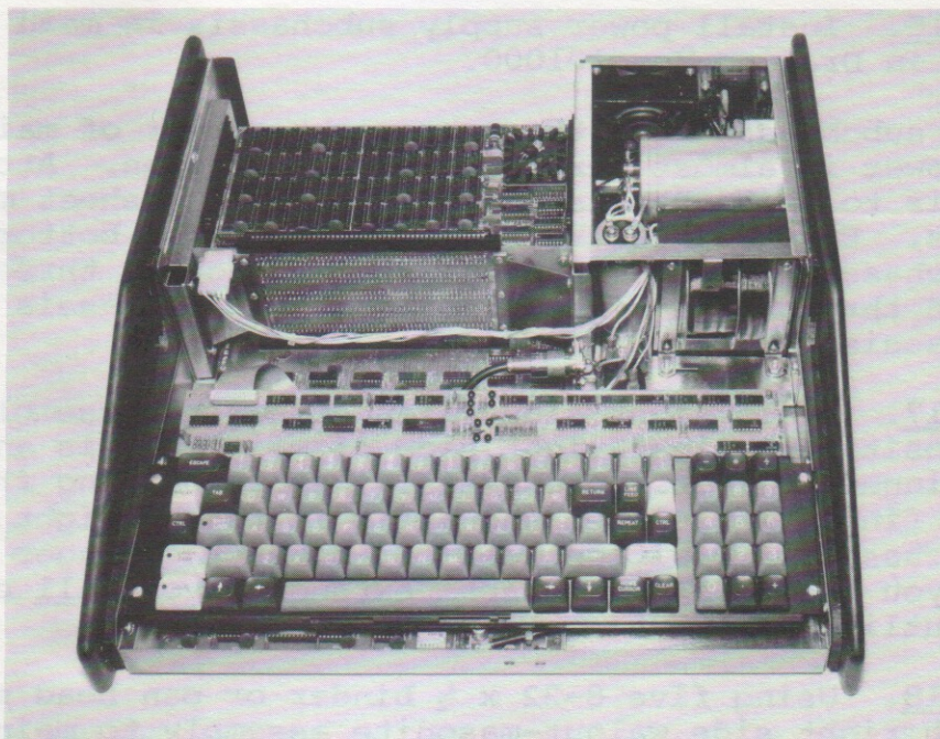
Figure 6-3. Sol-20 with covers removed. Front (or keyboard) is in foreground, power supply is in right rear corner, expansion chassis (with 8KRA Memory installed) is to left of power supply. The vertical board just behind white connector on left is the backplane board.
