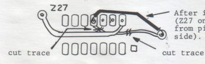
After installation of socket at U27 (Z27 on etch) install jumper wire from pin 11 to pad as shown (solder side).
