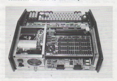
Figure 6-4. Sol-20 with covers removed. Rear side of assembly is in foreground and Sol-PC is just visible at lower right rear of assembly. 8KRA Memory is installed in expansion chassis above Sol-PC.
