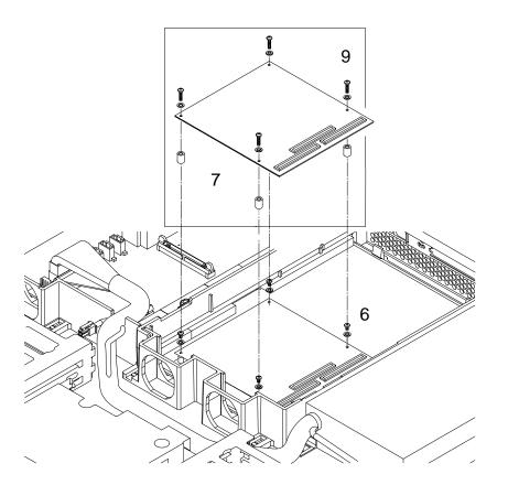
There is one memory board in the shipped system. You can upgrade it and install an additional memory board.
