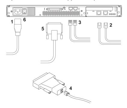
1 Connect the Netra t1 Model 105 AC power cord. 2 Connect the two Ethernet devices. 3 Connect up to two serial devices. You must connect a console to one serial port. You can also connect to the LOMlite device for remote power on/off via the port marked LOM/Serial A. See the Netra t1 LOMlite User's Guide for details. 4 If required, insert the serial cable for external devices into the adapter. 5 If required, connect a SCSI adapter to the SCSI cable. 6 Turn power supply switch on.
